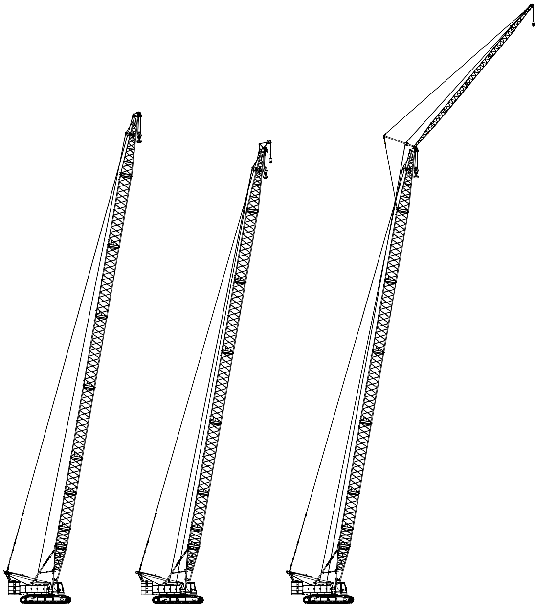
Operating condition of Main boom H (18~81)m (53+16)t
